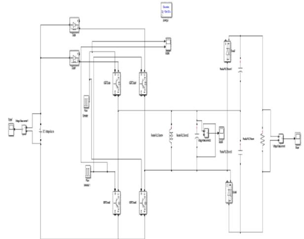
Fig:4.1 simulink diagram of step up resonant converter
