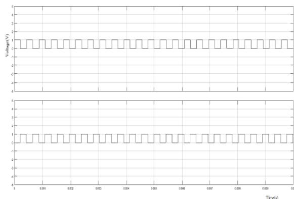
Fig 4. 2 pulses for switches Q1, Q4 and Q2, Q3.
