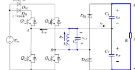
Fig:3.6 Equivalent circuit of mode 6
