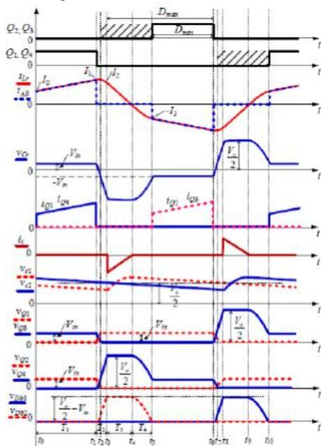
Fig:3.9 Operating waveforms of the proposed converter
