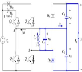
Fig:3.7 Equivalent circuit of mode 7
