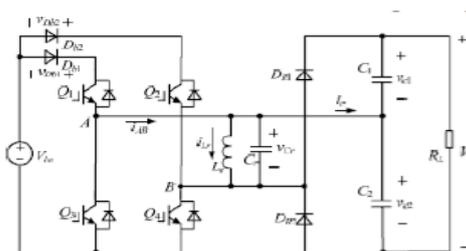
**Fig:2.1** Proposed step up resonant converter
