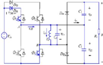
Fig:3.1 Equivalent circuit of mode 1
