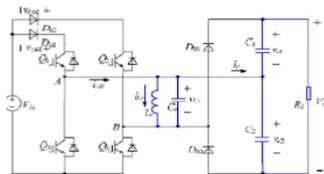
Fig:3.2 Equivalent circuit of mode 2
